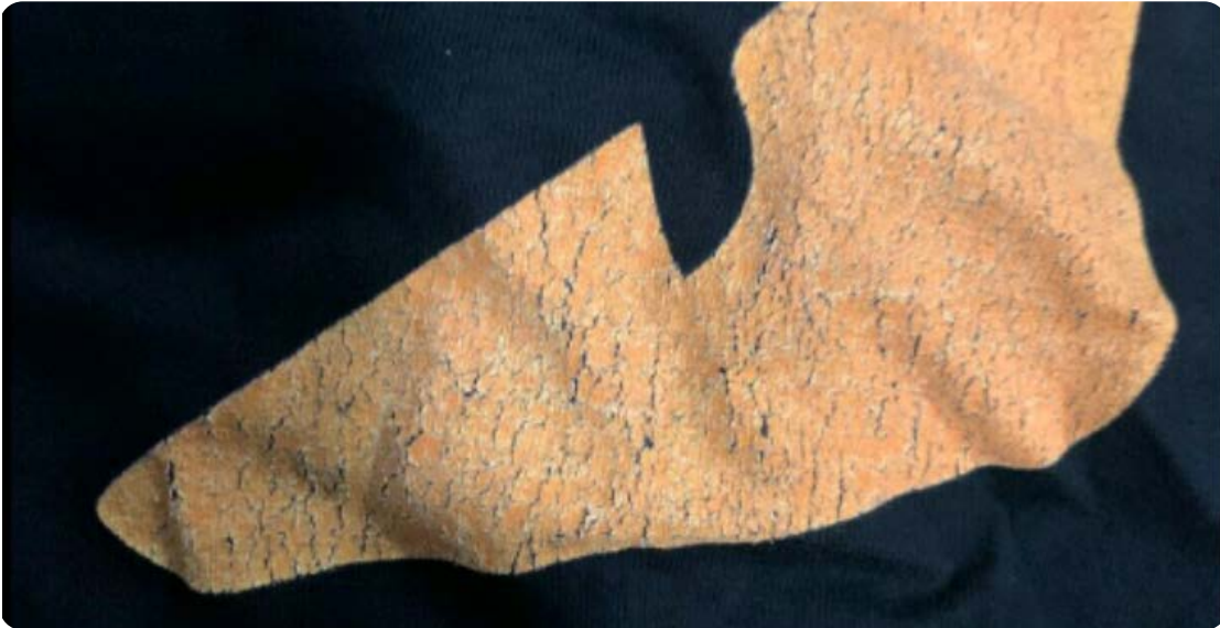
Cracks appearing after wash
